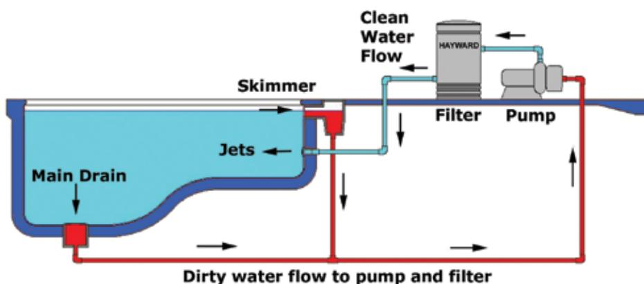
**Single Line Suction System** has a pipe that runs from the skimmer, connects with the main drain pipe, goes directly into the pump and filter, and then back into the pool.
