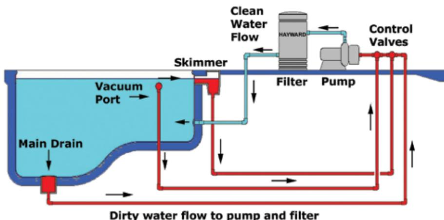
**Multi-port Suction System** has individual pipes running from the main drain and skimmer. These interconnect just before they reach the pump and typically have a valve that can be adjusted. This valve allows you to manipulate the force of suction from the skimmer or main drain. Some pools have a side port with an individual valve adjustment, which an automated floor vacuum can be attached. The side port pipe that leads to the pump is separate from the main drain and skimmer pipes.
